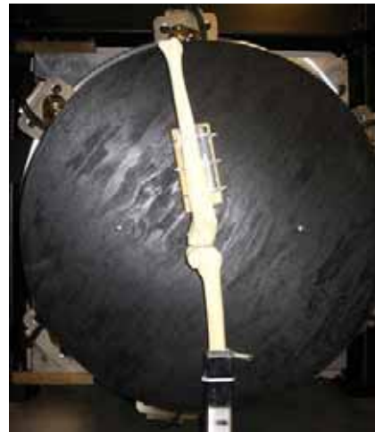
Figure 1: Testing set-up. Tibia is secured to the parallel robot (top) and the femur is grounded (bottom).
