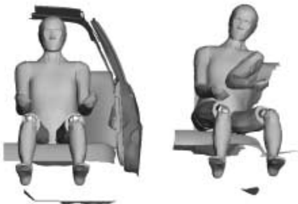
Figure 1: ESI H-Model in initial position (left) and during crash (right)
